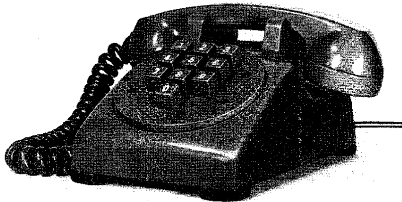
Fig. 1 — Modified 500-type telephone set equipped experimentally with tone ringer and pushbutton caller.
